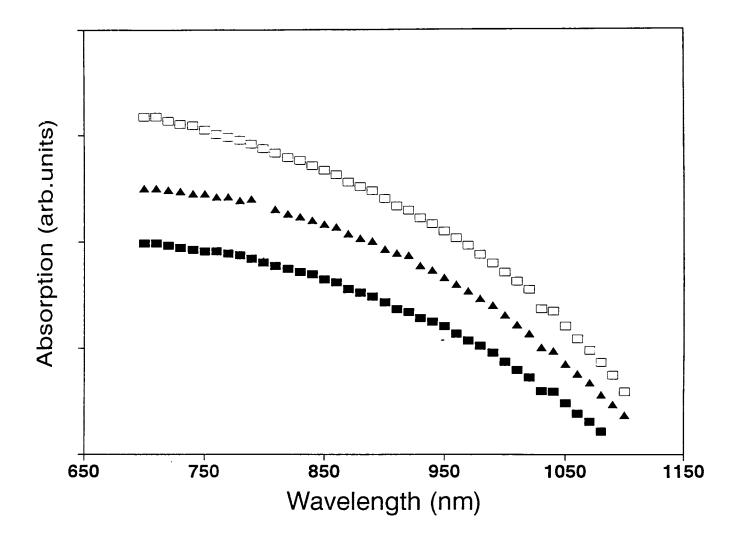
Fig. 6.4 UV-Vis - NIR spectra of  $Ge_{20}Bi_xSe_{80-x}$  glasses. ( $\blacksquare$ )Ge<sub>20</sub>Bi<sub>8</sub>Se<sub>72</sub> ( $\square$ ) Ge<sub>20</sub>Bi<sub>10</sub>Se<sub>70</sub> ( $\triangle$ )Ge<sub>20</sub>Bi<sub>12</sub>Se<sub>68</sub>.
