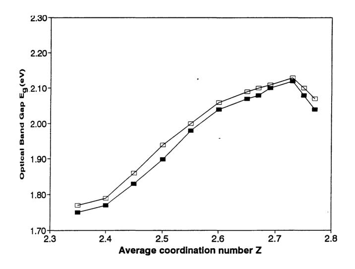
**Fig. 4.9** Variation of the optical band gap E<sub>g</sub> with average coordination number Z for the Ge<sub>x</sub>Ga<sub>5</sub>Se<sub>95-x</sub> glasses using PA technique (□) and UV-Vis-NIR absorption technique (■).
