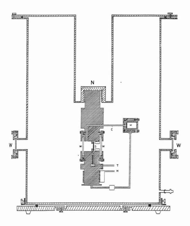
Fig. 3.4 Schematic diagram of the variable temperature PA cell.
