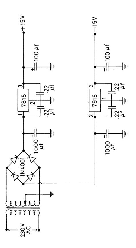
Fig. 2.7 Schematic diagram of the power supply.
