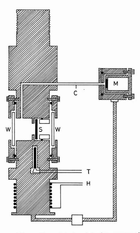
Fig. 3.3 Schematic diagram of the sample chamber and microphone compartment. W- cell windows, S- sample, C- coupling tube, M- microphone, T- temperature sensor, H - heater winding.
