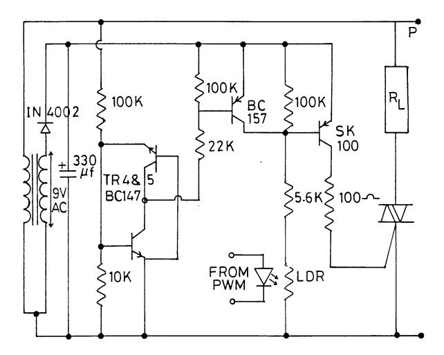
Fig. 2.6 Schematic diagram of solid state relay.
