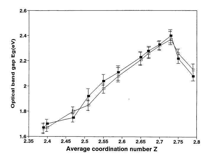
Fig. 5.8 Variation of the optical band gap E<sub>g</sub> with average coordination number Z for the Ge<sub>x</sub>In<sub>5</sub>Se<sub>95-x</sub> glasses using PA technique (■) and UV-Vis-NIR absorption technique (□).
