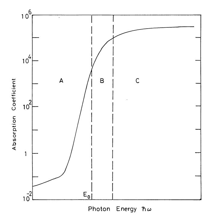
Fig. 1.4 Schematic representation of the absorption spectrum of amorphous semiconductors showing three different regions A, B and C.
