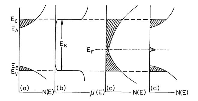
Fig.1.3 Density of states and mobility as a function of energy in amorphous semiconductors.
