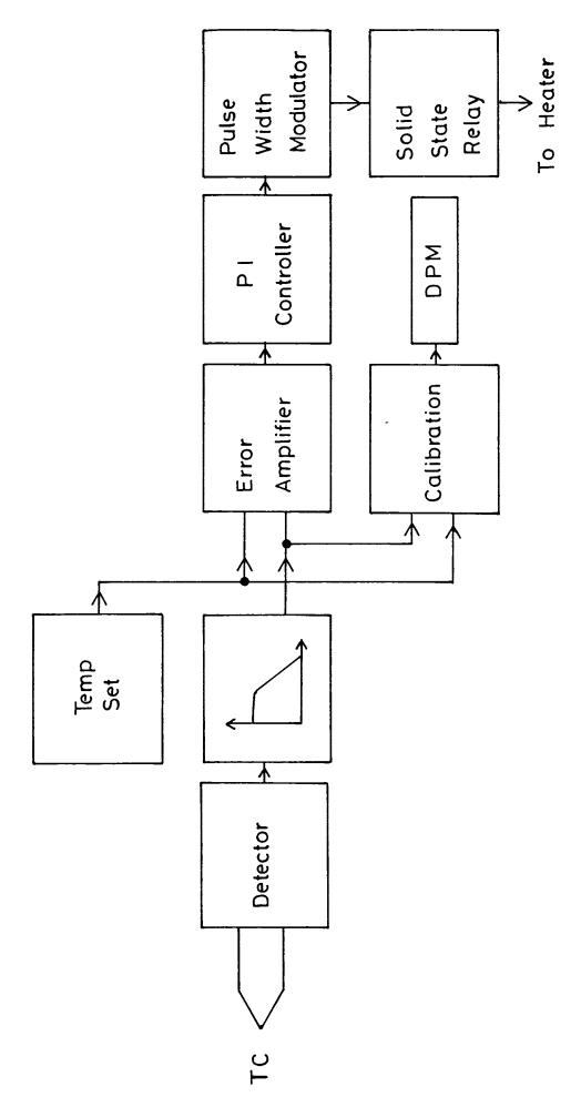
Fig. 2.3 Block diagram of the temperature controller.
