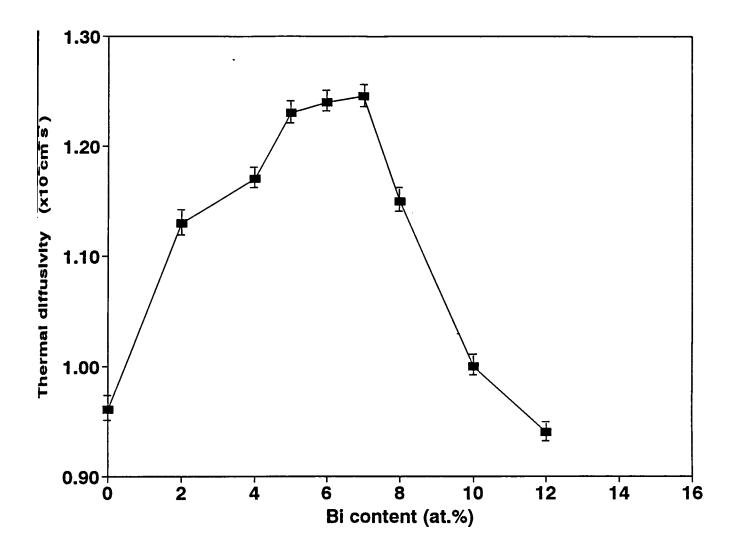
Fig. 6.6 Variation of thermal diffusivity  $\alpha$  with average coordination number Z for Ge<sub>20</sub>Bi<sub>x</sub>Se<sub>80-x</sub> glasses.
