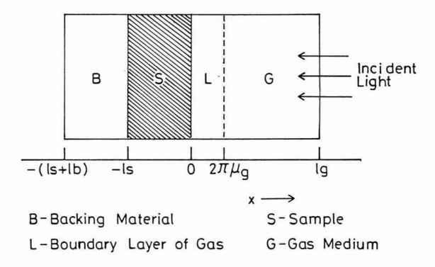
Fig. 1.1 Cross-sectional view of a simple cylindrical PA cell.
