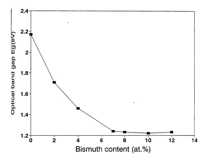
Fig. 6.5 Variation of the optical band gap Eg with average coordination number Z for the  $Ge_{20}Bi_xSe_{80-x}$  glasses using UV-Vis-NIR absorption technique.
