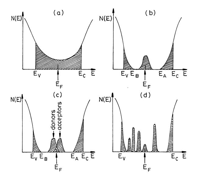
Fig. 1.2 Schematic density of states diagram for amorphous semiconductors(a) The CFO model (b) Davis- Mott model showing a band of compensated levels near the middle of the gap (c) modified Davis-Mott model(d) the "real" glass with defect states.
