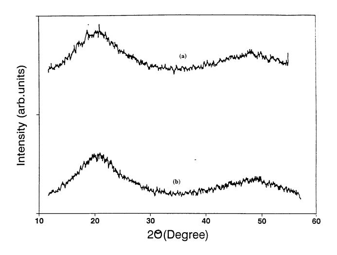
Fig. 4.1 X- ray diffraction pattern of (a)  $Ge_{12.5}Ga_5Se_{82.5}$  and (b)  $Ge_{26}Ga_5Se_{69}$  glasses.
