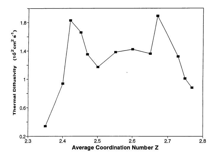
Fig. 4.10 Variation of thermal diffusivity  $\alpha$  with average coordination number Z for  $Ge_xGa_5Se_{95-x}$  glasses.
