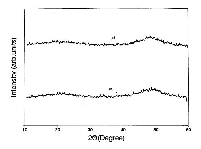
Fig. 6.1 X- ray diffraction pattern of (a) $Ge_{20}Bi_5Se_{75}$  and (b) $Ge_{20}Bi_{10}Se_{70}$  glasses.
