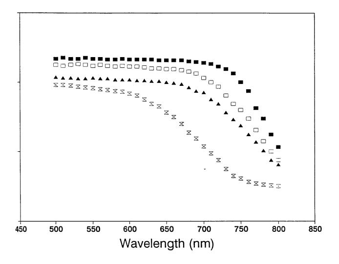
Fig. 5.3 PA spectra of Ge  $_x$  In<sub>5</sub> Se<sub>95-x</sub> glasses. ( $\blacksquare$ ) Ge<sub>12</sub>In<sub>5</sub>Se<sub>83</sub> ( $\square$ ) Ge<sub>13</sub>In<sub>5</sub>Se<sub>82</sub> ( $\blacktriangle$ ) Ge<sub>16</sub>In<sub>5</sub>Se<sub>79</sub> ( $\Chi$ ) Ge<sub>18</sub>In<sub>5</sub>Se<sub>77</sub>.
