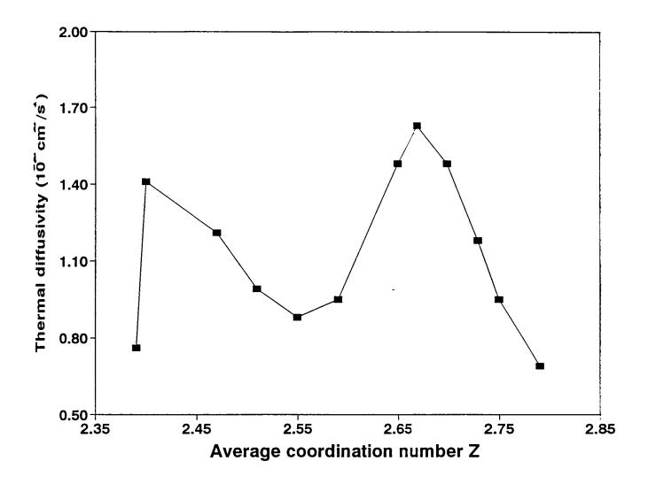
Fig. 5.9 Variation of thermal diffusivity  $\alpha$  with average coordination number Z for Ge<sub>x</sub>In<sub>5</sub>Se<sub>95-x</sub> glasses.
