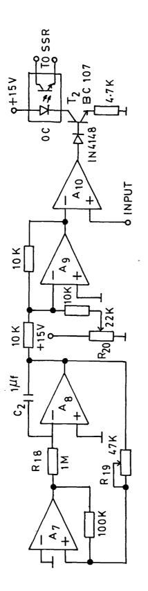
Fig. 2.5 Schematic diagram of pulse width modulator. A<sub>7</sub> - A<sub>10</sub> LM 324 quad. op. amp., OC -optocoupler.
