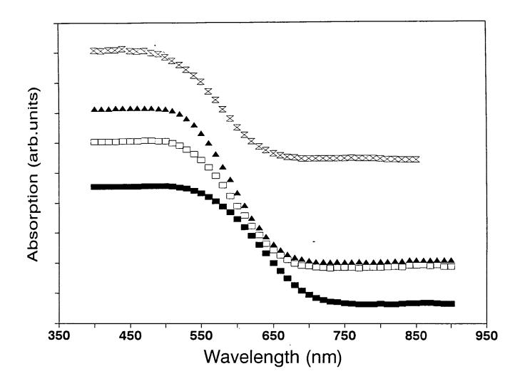
Fig. 5.6 UV-Vis - NIR spectra of  $Ge_xIn_5Se_{95-x}$  glasses. ( $\blacksquare$ )Ge\_{22}In\_5Se\_{73} ( $\square$ ) Ge\_{25}In\_5Se\_{70} ( $\blacktriangle$ )Ge\_{26}In\_5Se\_{69} (X) Ge<sub>28</sub>In<sub>5</sub>Se<sub>67</sub>.
