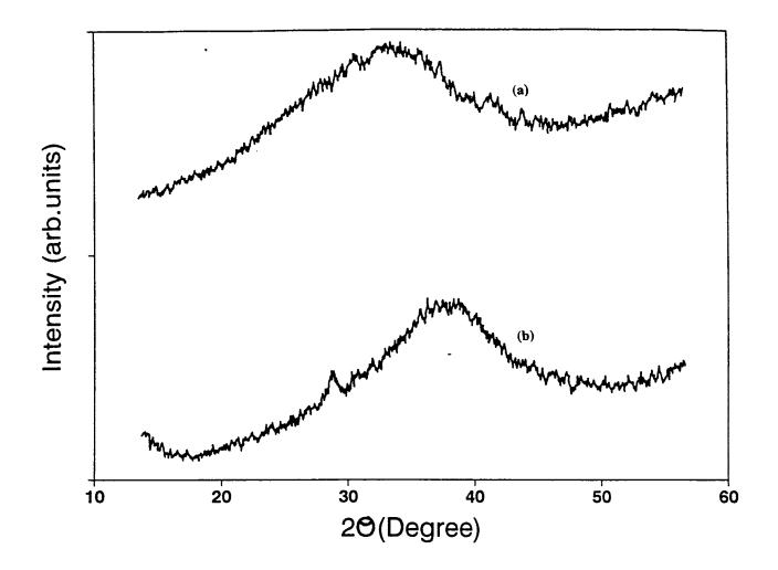
Fig. 5.1 X- ray diffraction pattern of (a)  $Ge_{13}In_5Se_{82}$  and (b)  $Ge_{26}In_5Se_{69}$  glasses.
