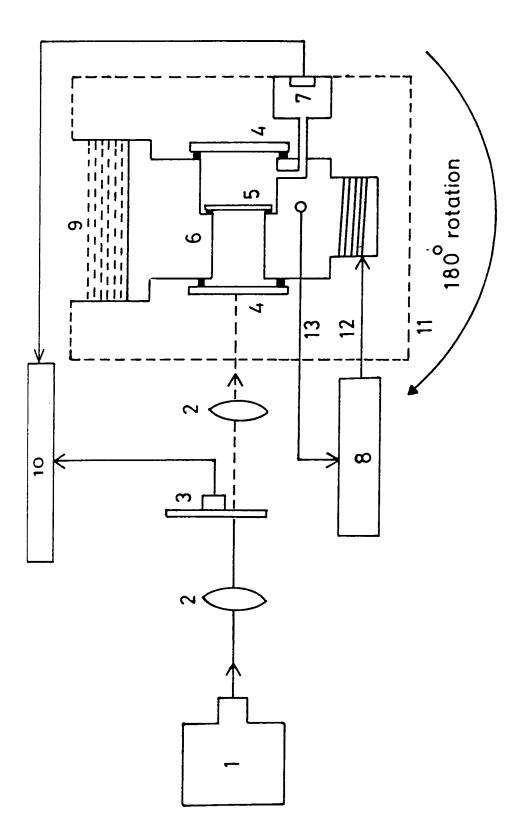
4-cell windows, 5- sample, 6- sample holder, 7- microphone, 8-temperature controller, Fig. 3.2 Schematic diagram of the experimental set up. 1-source, 2- lenses, 3- chopper, 9- liquid nitrogen chamber, 10- lock-in amplifier, 11- outer chamber, 12- heater, 13- temperature sensor.
