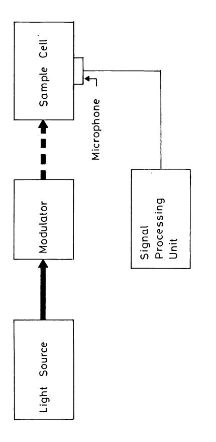
Fig. 2.1 Basic set up of a gas - microphone PA spectrometer.
