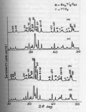
Figure 3 X-ray diffraction (XRD) patterns of typical 115 ceramics (a) La-compound, (b) La-compound with 5%  $Bi_2O_3$  added (c) Nd-compound and (d) Nd-compound with 5%  $Bi_2O_3$  added.
