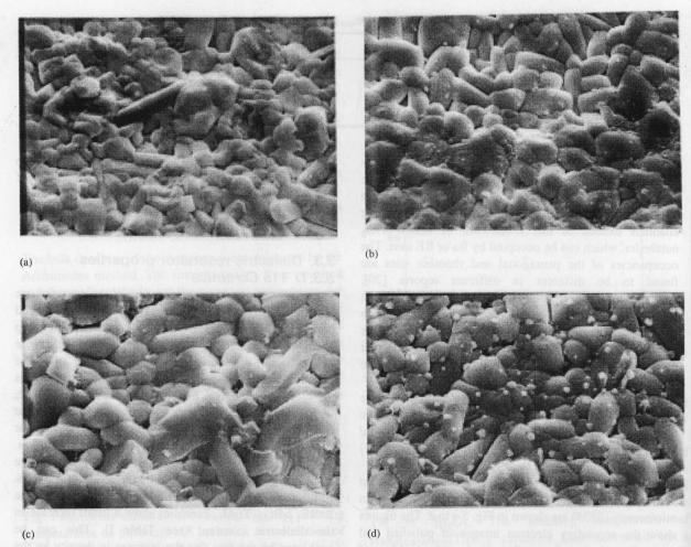
Figure 5 Secondary electron images of the etched surfaces of 115 ceramics (a) Nd-compound (b) Nd-compound with 10%  $Bi_2O_3$  added. Similar images obtained for 114 ceramics (c) Nd-compound, (d) Nd-compound with 10%  $Bi_2O_3$  added.
