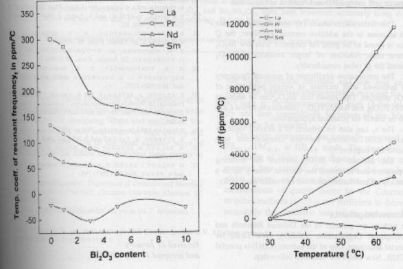
Figure 10 Effect of  $Bi_2O_3$  addition on the temperature coefficient of resonant frequencies ( $\tau$ ) of 114 ceramics.
