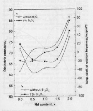
*Figure 8* Influence of substitution (*x*) and Bi<sub>2</sub>O<sub>3</sub> addition on the dielectric constants ( $\varepsilon_r$ ) of Ba(Nd<sub>x</sub>Sm<sub>2-x</sub>)Ti<sub>5</sub>O<sub>14</sub> ceramics.
