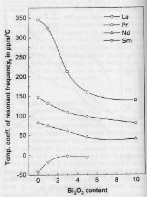
Figure 9 Effect of  $Bi_2O_3$  addition on the temperature coefficient of resonant frequencies ( $\tau_f$ ) of 115 ceramics.
