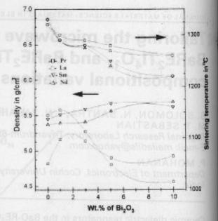
*Figure 2* Variation of bulk densities and sintering temperatures of 114 ceramics due to the addition of  $Bi_2O_3$ .
