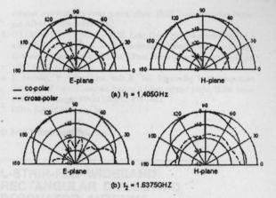
**Figure 4** Measured E- and H-plane radiation patterns of the antenna at  $f_1 = 1.405$  GHz and  $f_2 = 1.6375$  GHz for V = -19 V
