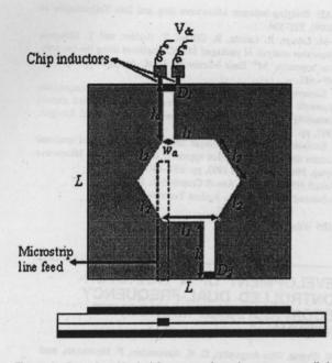
Figure 1 Reconfigurable dual-frequency microstrip antenna controlled by varactor diodes. (antenna parameters are given in Fig. 2)
