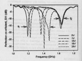
**Figure 2** Measured reflection coefficient  $(S_{11})$  of the antenna for different varactor reverse-bias voltages  $(L = 4 \text{ cm}, l_1 = l_2 = 0.8 \text{ cm}, l_a = l_b = 1.1 \text{ cm}, w_a = 0.1 \text{ cm}, h = 0.16 \text{ cm}, \text{ and } \varepsilon_r = 3.98)$
