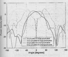
Figure 4 Measured H-plane radiation patterns
