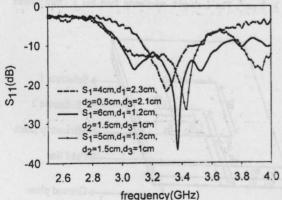
**Figure 2** Variation of  $S_{11}$  with frequency for different feed lengths of the antenna ( $h_1 = h_2 = 0.16$  cm,  $\varepsilon_{r1} = \varepsilon_{r2} = 4.28$ , L = 4 cm, W = 2 cm,  $S_2 = 3.5$  cm)
