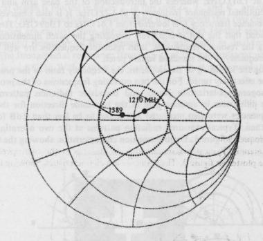
Figure 5. Measured input impedance on a smith chart for the proposed antenna.
