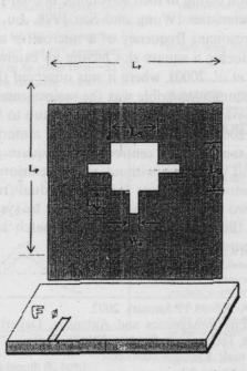
Figure 1. Geometry of the proposed dual-frequency dual-polarized slotted square microstrip antenna.
