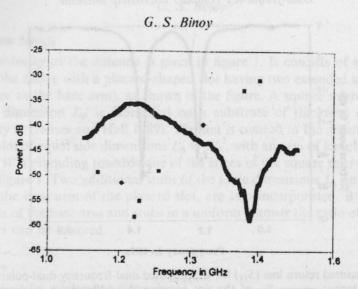
Figure 4. Variation of received power with frequency for the two orthogonal polarization planes: ...... vertical polarization; —— horizontal polarization.
