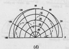
Figure 3 Radiation pattern of the antenna for the two resonant frequencies. (a) *H*-plane patterns for 1.593 GHz. (b) *E*-plane patterns for 1.593 GHz. (c) *H*-plane patterns for 1.797 GHz. (d) *E*-plane patterns for 1.797 GHz. — copolar, --- cross polar
