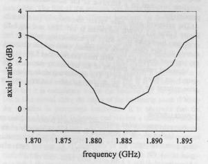
Figure 3 Measured axial ratio against frequency
